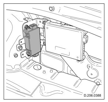
Fig. 19 Parking brake module
