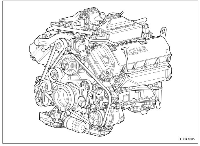
Fig. 32 V8 supercharged engine
