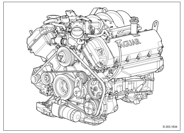
Fig. 31 V8 normally aspirated engine
