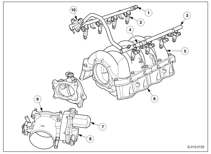
Fig. 47 Fuel charging system — V8 normally aspirated
