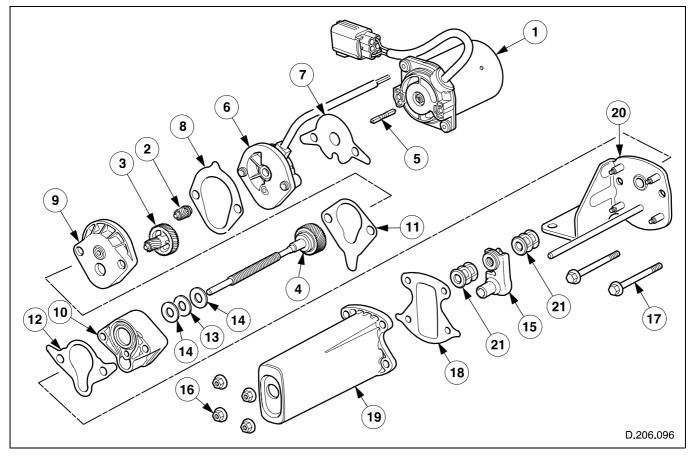
Fig. 21 Motorized actuator unit — internals
