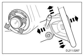
Fig. 27 Steering column adjustment
