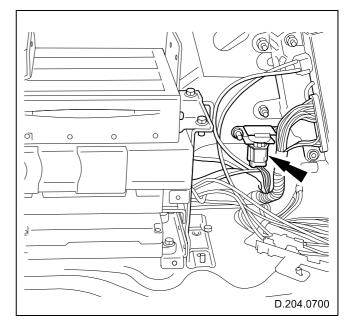
Fig. 13 Rear vertical accelerometer
