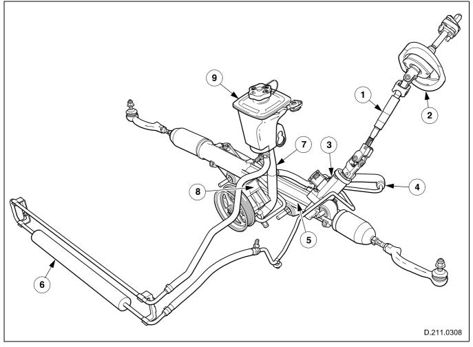
Fig. 25 Steering system assembly – V8 derivative shown
