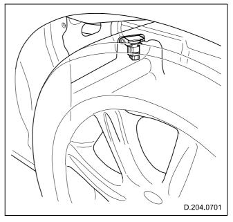
Fig. 12 Front vertical accelerometer
