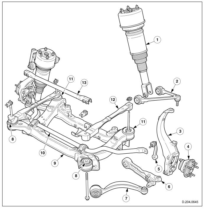
Fig. 2 Front suspension components
