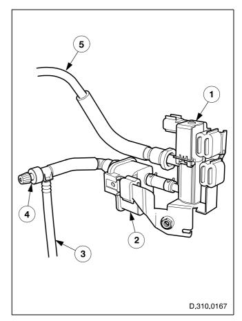
Fig. 50 Evaporative emission canister purge valve
