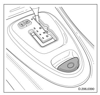
Fig. 18 Parking brake switch
