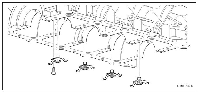
Fig. 33 Piston cooling jets - supercharged engine only
