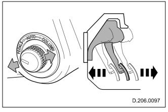
Pedal adjustment is enabled by setting the 3-way, rotary switch situated on the left-hand side of the steering column, to the appropriate position. Pedal adjustment is then controlled by operating the switch upwards, for pedals 'out' and downwards for pedals 'in'.
