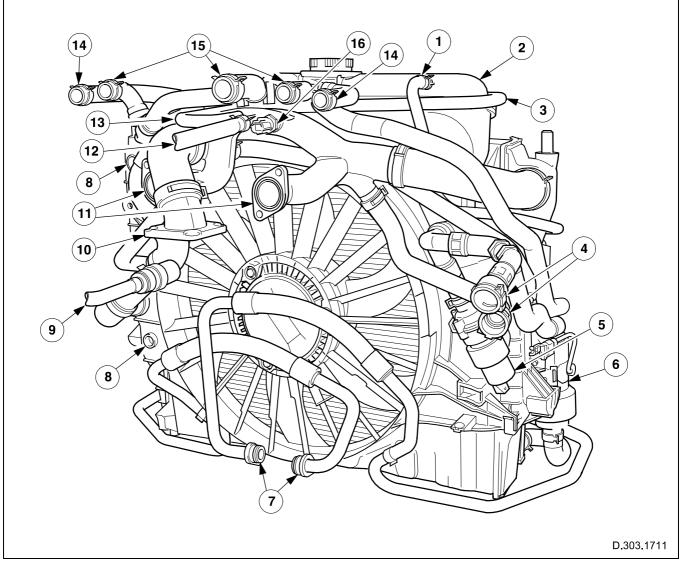
Fig. 43 V8 SC cooling system components and connections
