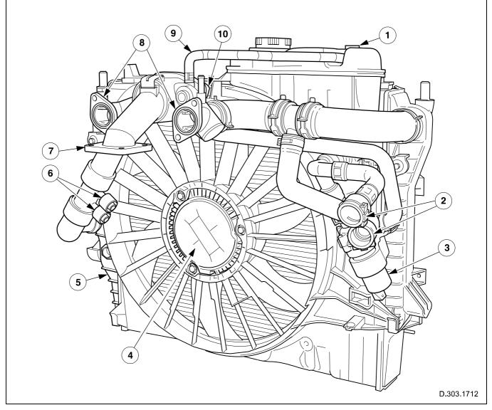
Fig. 41 V8 cooling system components and connections
