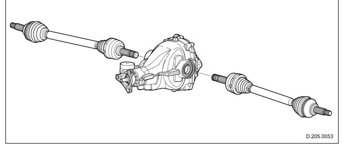
Fig. 15 Axle shafts and final drive unit
