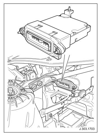
Fig. 51 Engine control module
