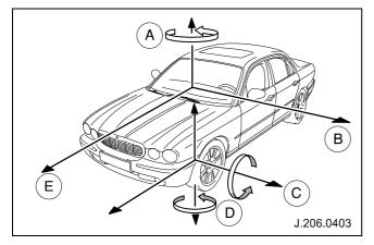
Fig. 17 Vehicle travel directions
