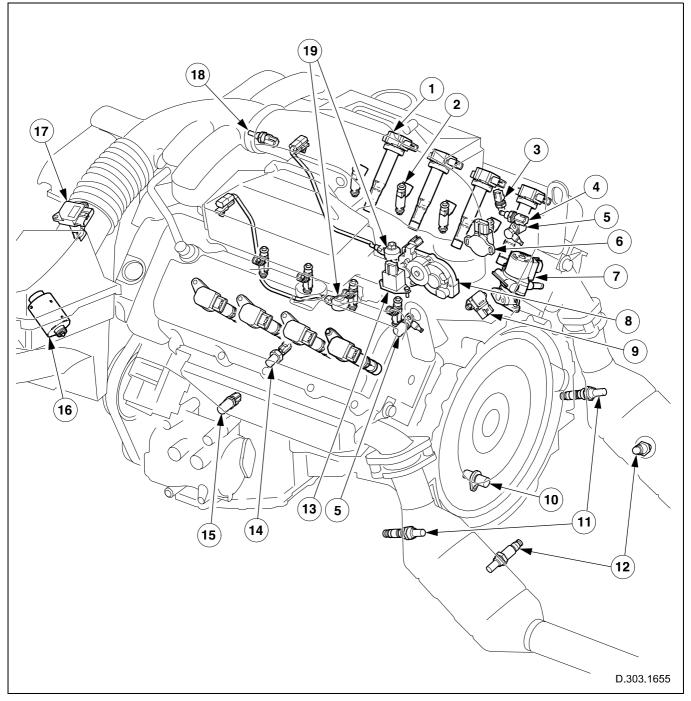
Fig. 57 V8 supercharged Engine — sensor and actuator location
