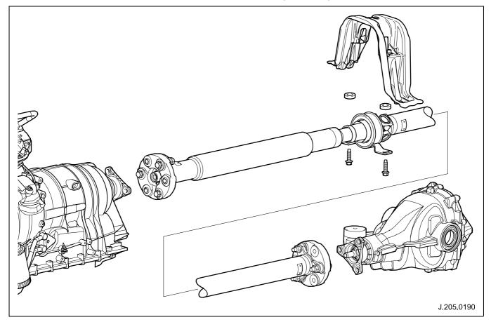
Fig. 14 Driveshaft and final drive unit
