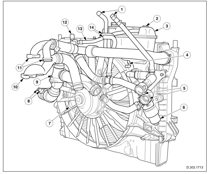
Fig. 39 V6 cooling system components and connections (4-zone climate control variant)
