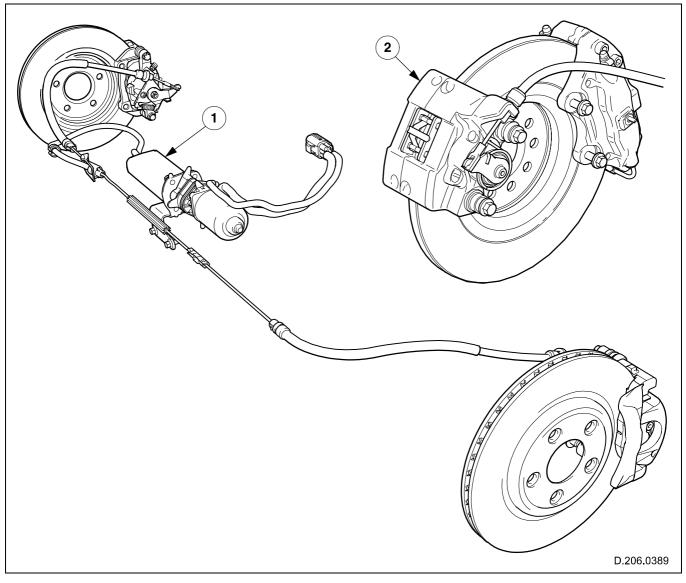
Fig. 20 Actuator unit and cables
