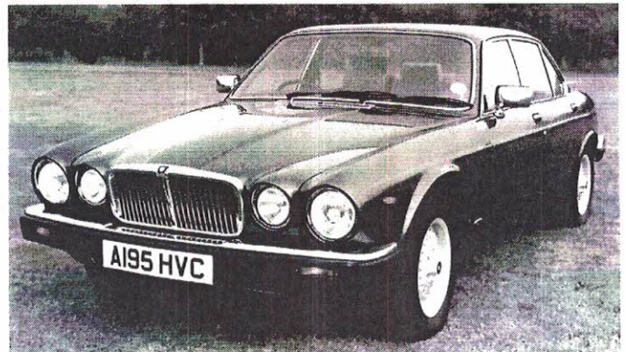
Jaguar Sovereign HE – Front view showing the Pepperpot Alloy Wheels and headlamp wash/wipe.
