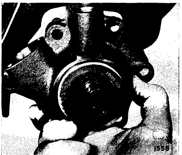
Fig. 100. Fitting the bearing retainer.
