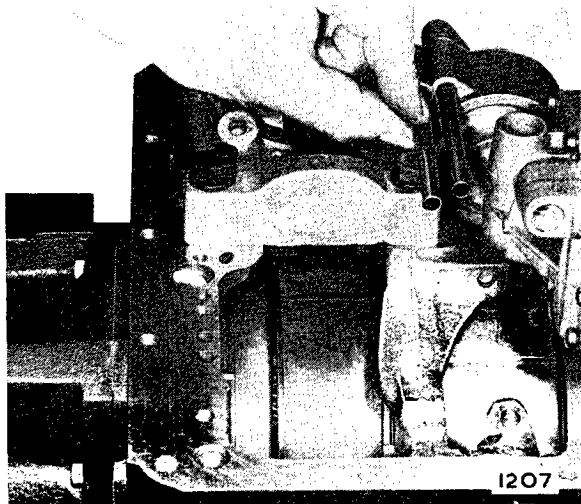
Fig. 22. Withdrawing the apply and release tubes.
