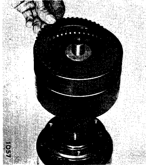
Fig. 58. Fitting a front clutch outer plate.
