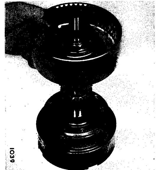
Fig. 47. Fitting the rear clutch piston and cylinder.
