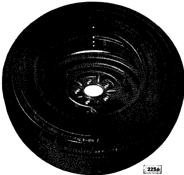
Fig. 3. Correct position of the inner tube to outer cover to facilitate wheel balance
