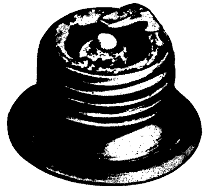
Fig. 50. Badly burned sparking plug
