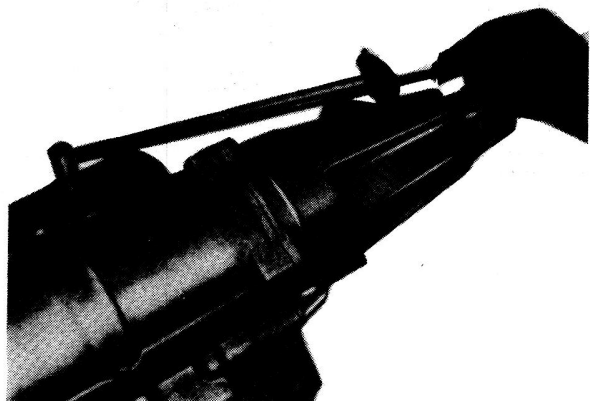
Fig.6.47. Adjusting the rear brake band
