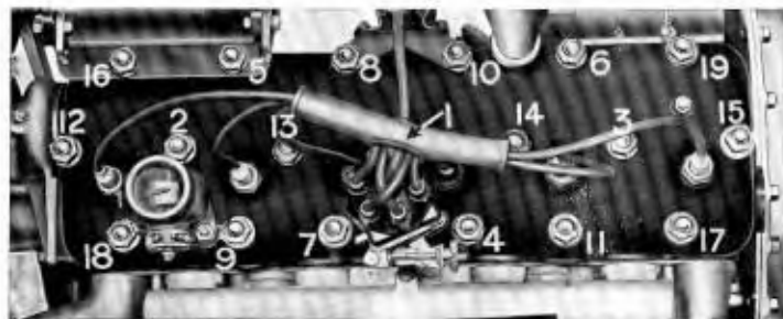
Fig. 30. S.S. I. Correct order for tightening the Cylinder Head Nuts.
