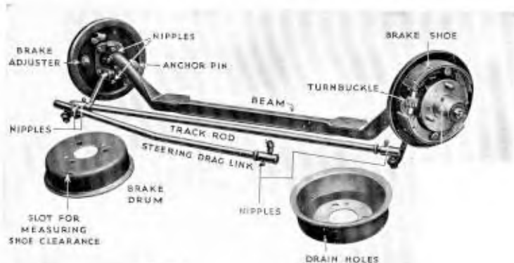
Fig. 12. Front Axle and Brake Details.
