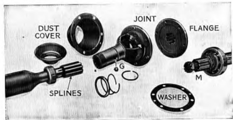
View of Universal Joint dismantled. M—Gearbox mainshaft.
