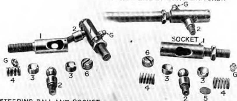
STEERING BALL AND SOCKET TWO ON TRACK ROD ONE ON STEERING END OF DRAG LINK.
