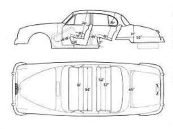
BODY. All steel, four door, five-seater Sedan. Integral bodychassis construction providing maximum rigidity with minimum
